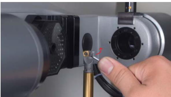
Direction to increase boring diameter.
